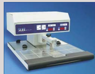
MPS/P1 with preheat areas, dispenser and cold spot
