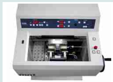
MNT chamber and controller
